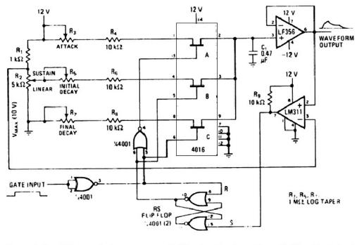
generator provides myriad control waveforms for modulating voltage-controlled amplifiers, oscillators, and filters in a music synthesizer, and thus is useful for coloring loudness, pitch, and timbre. Attack and decay times are variable from 5 to 500 milliseconds; sustain level is adjustable from 0 to 10 volts.
